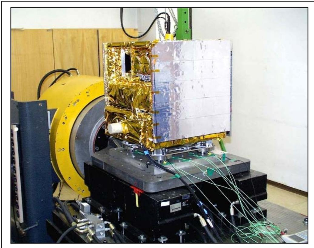
**Figure 3** BIRD with solar array on vibration test bench
