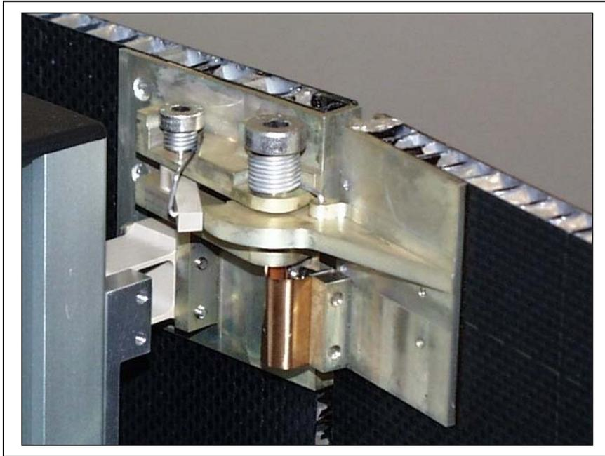
**Figure 2** Joint with drive spring, locking latch and grounding plate
